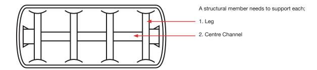
2. Bolt the tank legs to the skid or deck
